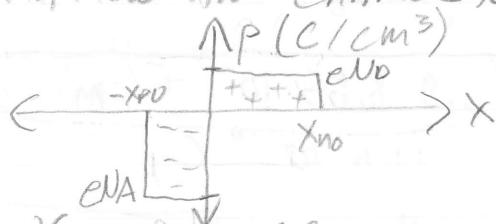
$$\frac{\partial E}{\partial x} = \frac{f}{E} = \begin{cases} -\frac{e}{E} N_A & \text{FOR } -x_{p0} < x < 0 \\ \frac{e}{E} N_D & \text{FOR } 0 < x < x_{n0} \end{cases}$$
