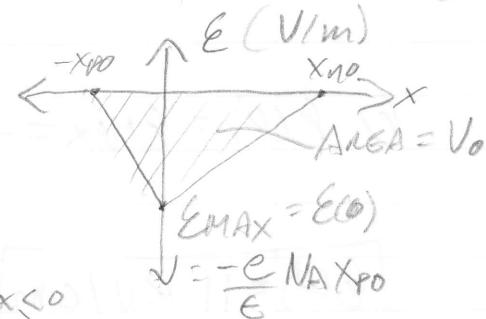
$$E = -\frac{dV}{dx} \Rightarrow V = \begin{cases} \frac{-eN_A x_{p0}^2}{2E} & x \leq -x_{p0} \\ \frac{eN_A (\frac{1}{2}x^2 + x \cdot x_{p0})}{2E} & -x_{p0} < x < 0 \\ \frac{-eN_D (\frac{1}{2}x^2 - x \cdot x_{n0})}{2E} & 0 < x < x_{n0} \\ \frac{eN_D x_{n0}^2}{2E} & x \geq x_{n0} \end{cases}$$
